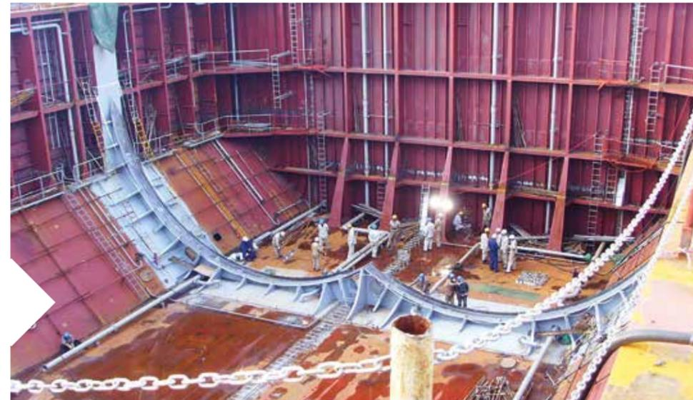
Cargo hold structure of ECOSTAR 36k during construction at Dayang Shipyard, China.
