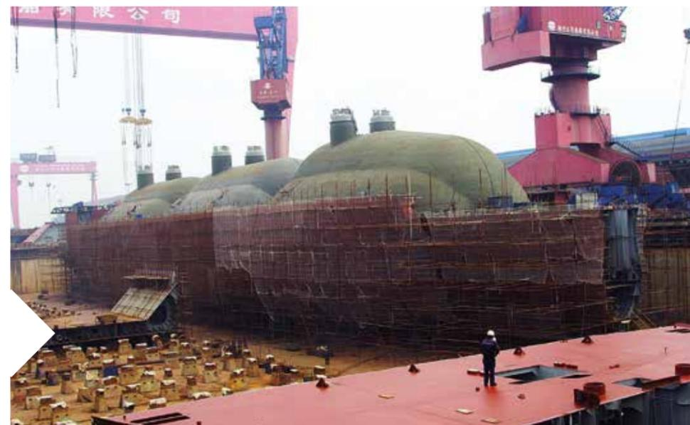
Cargo hold structure of ECOSTAR 36k with Star-Trilobe tanks installed. One cargo tank per day was mounted trouble-free.
