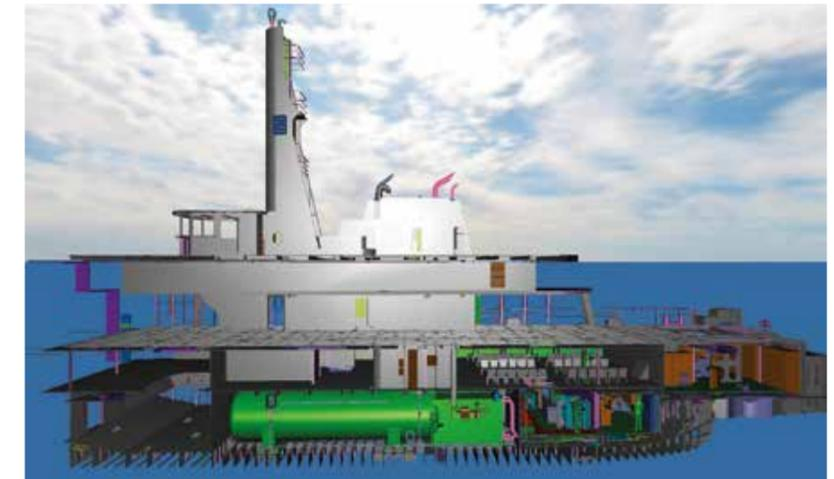
3D coordination model side view showing the fuel gas tank and fuel gas system
